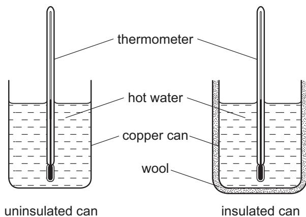
One can is insulated with wool. The temperature of the water in each can is taken every minute for several minutes. Graphs of the results are plotted.
